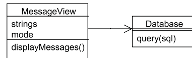
Figure 2.1 UML class diagram of the MessageView class with attributes, and the related Database class
