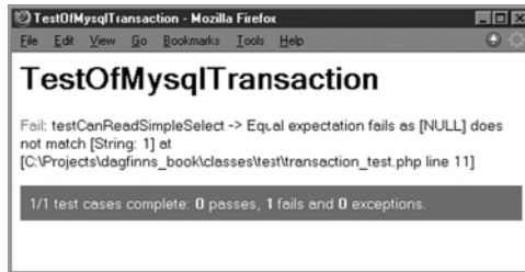
Figure 9.5 The test case no longer crashes, but the test fails since the code is not fully functional yet.
