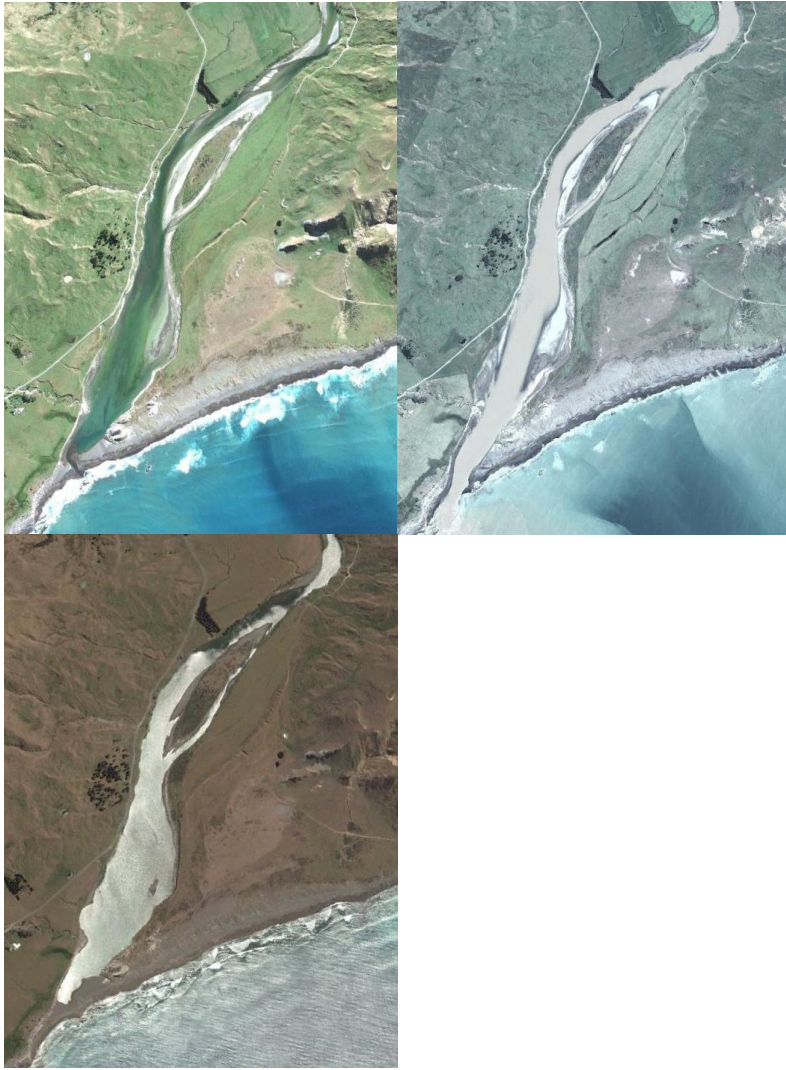
Figure 6-7: Pahaoa River, NZCHS type 6C tidal river mouth – barrier beach enclosed, showing changes in mouth openings that trap or release fine sediment. Images from 25 Mar 2010, 10 Jan 2012, 19 Feb 2016.
