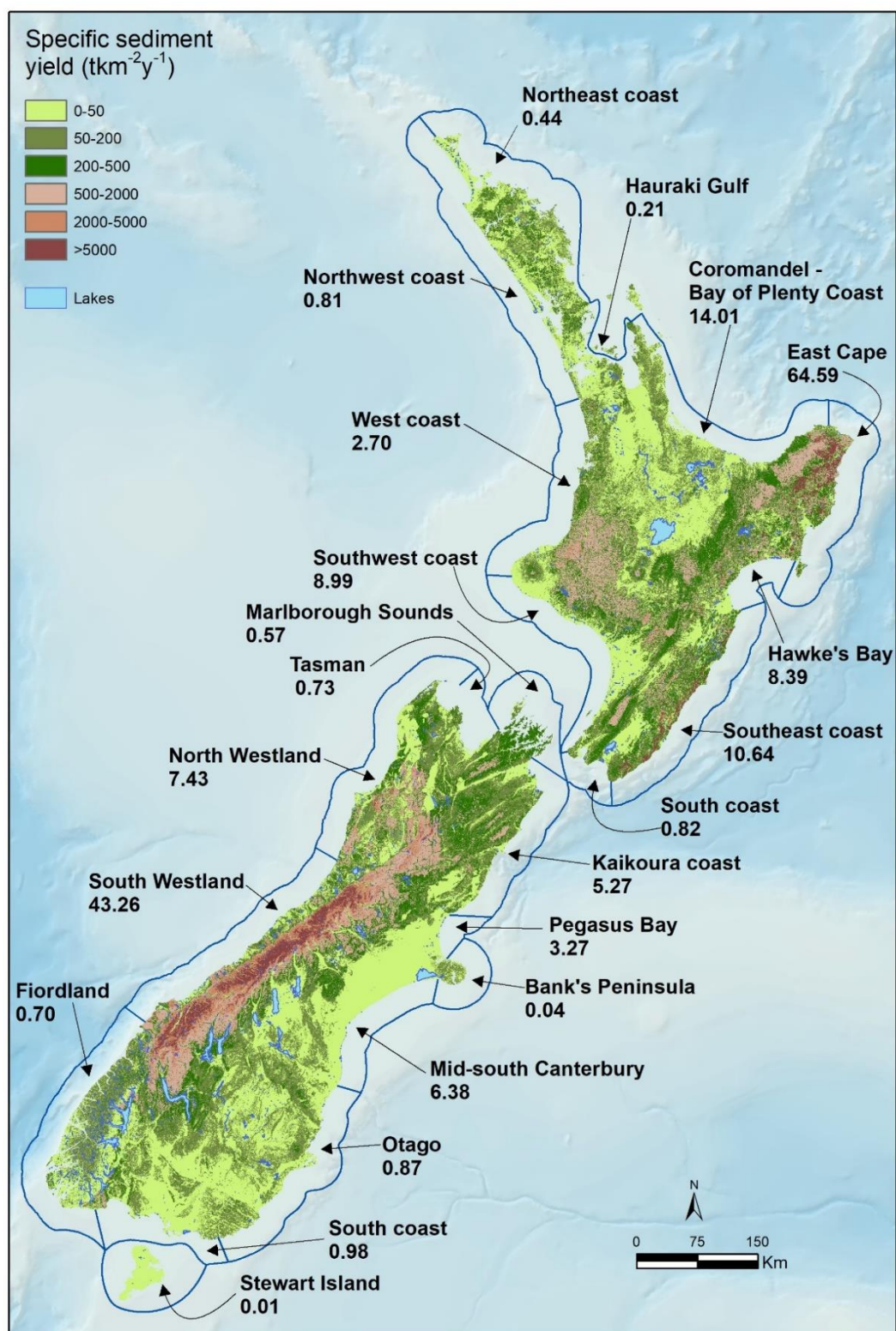
Figure 5-1: Specific yield map and load to the coast for current land cover. Sediment loads ( \text{Mt/y} ) delivered to the coast are totalled by coastal region. Coastal region boundaries are the same as in Hicks et al. (2011) and are defined on an arbitrary basis.
