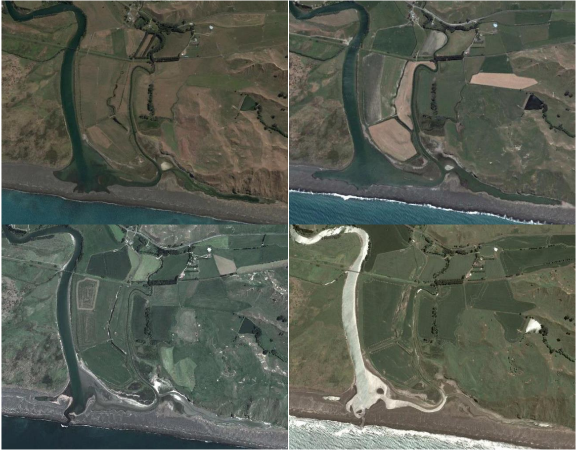
Figure 6-6: Nuhaka River, NZCHS type 4C beach stream – stream with pond, showing changes in mouth opening and pond size that trap or release fine sediments. Images from (top row) 2 Feb 2003, 24 Nov 2006, (bottom row) 12 Feb 2011 and 30 Dec 2013.
