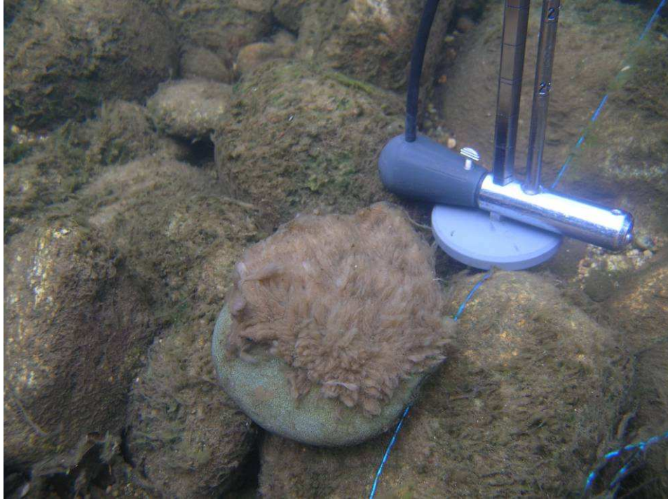
Measuring water depth and velocity of cobble substrates (longer-term trial) in the Monowai River (Stage 1).
