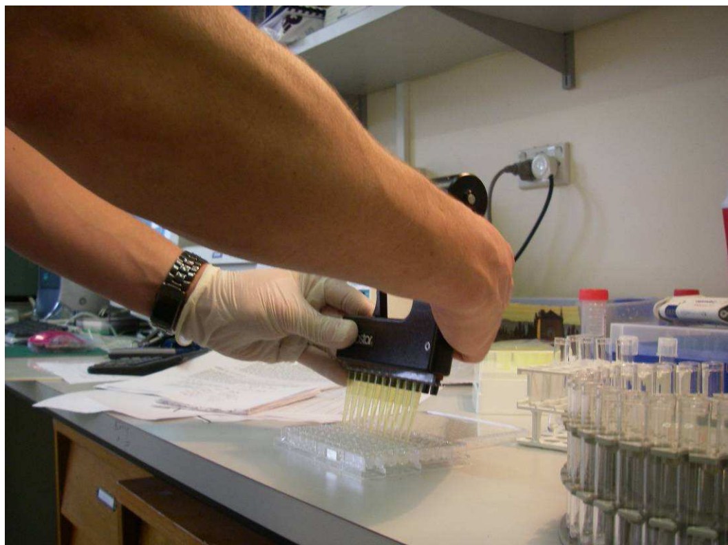
A multi-pipettor being used for sampling during toxicity testing in Hamilton (Stage 2 Phase 1).
