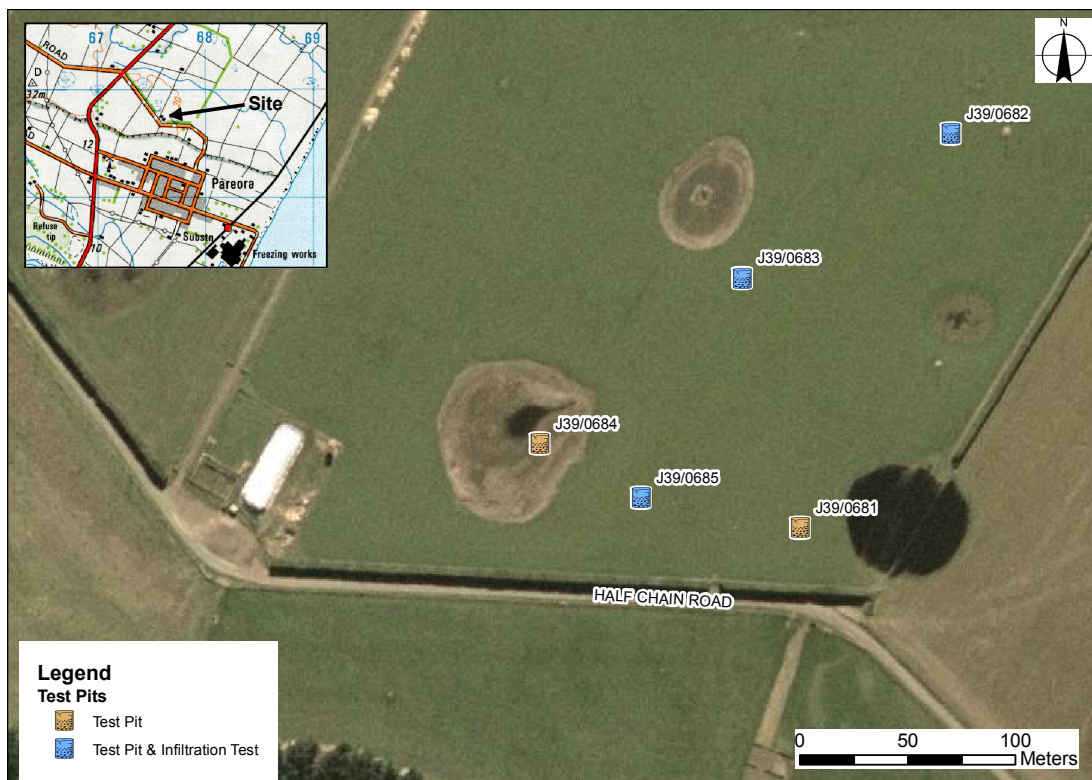
Figure 2: Map showing locations of test pits and those test pits within which infiltration tests were conducted. The sub-circular features shown in the aerial photograph are topographically isolated depressions that have swamps developed within these areas. These depressions do not have natural channel outlets although culverts now drain these areas.
