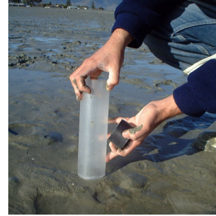
The perspex corer used to sample sediments.
