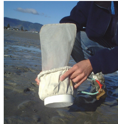
The PVC corer with 0.5 mm mesh bag attached for sampling infauna.
