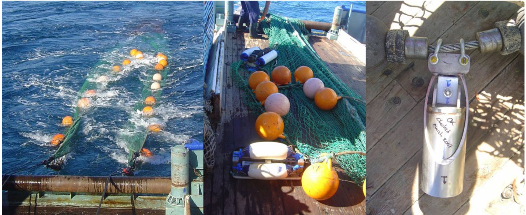
Figure A1.6: Headline deployed (left), showing CTD and contact sensor (middle) and bottom contact sensor attachment on groundrope (right).
