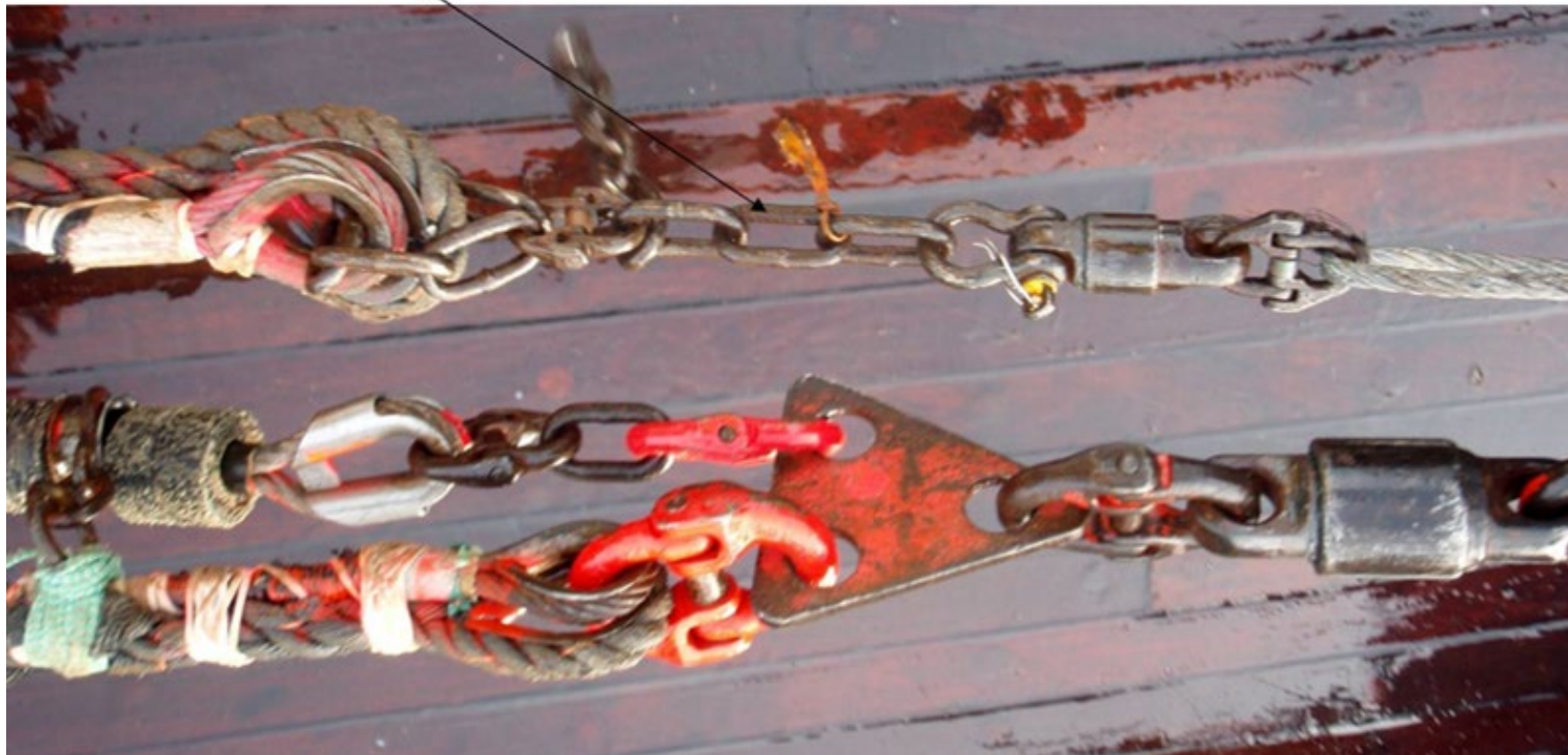
Figure A1.10: Top and bottom bridle-net attachments.
