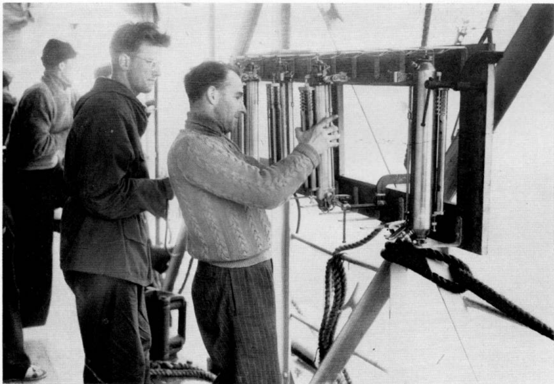
Plate 2. Reading reversing thermometers on board HMNZS Pukaki
