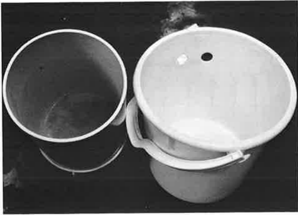
Figure 6: Bucket sieve. We use a 30 cm long piece of 20 cm diameter pipe with 80 µm mesh on one end. It sits inside a 20 l bucket with holes cut in the side to regulate the water level. The volume of water in the sieve when placed in the full bucket is 10 l.
