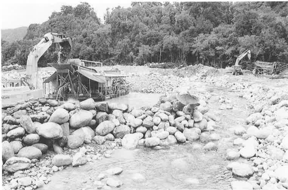
FIGURE 3. Mining machinery in operation, Big Hohonu River, August 1987. Note the clear water in the channel in the foreground. There was some leaching of coloured water from the dredge ponds through the tailings to the stream channel lower down but it was not considered to be excessive.
