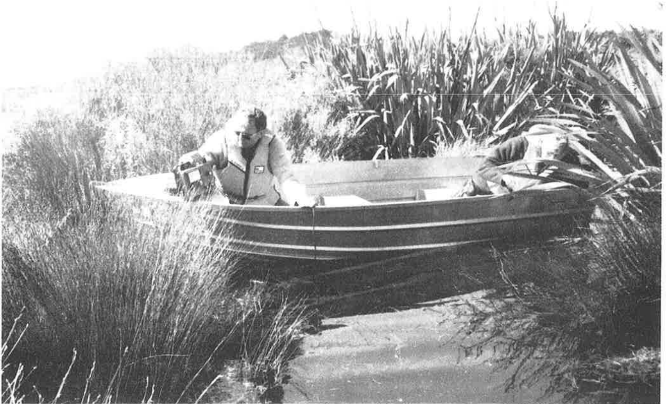
FIGURE 1. Using a salinometer to detect the saltwater wedge.
