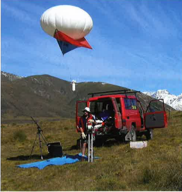
Tony Bromley sends up the Helikite near Lake Tennyson to record a vertical profile of wind and temperature.
