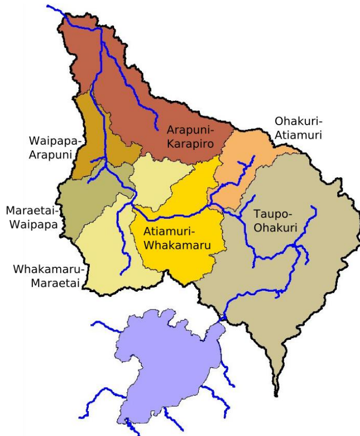
Figure 2 Separation of the upper Waikato catchment into the seven dam sub-catchments considered in the hydrological analysis
