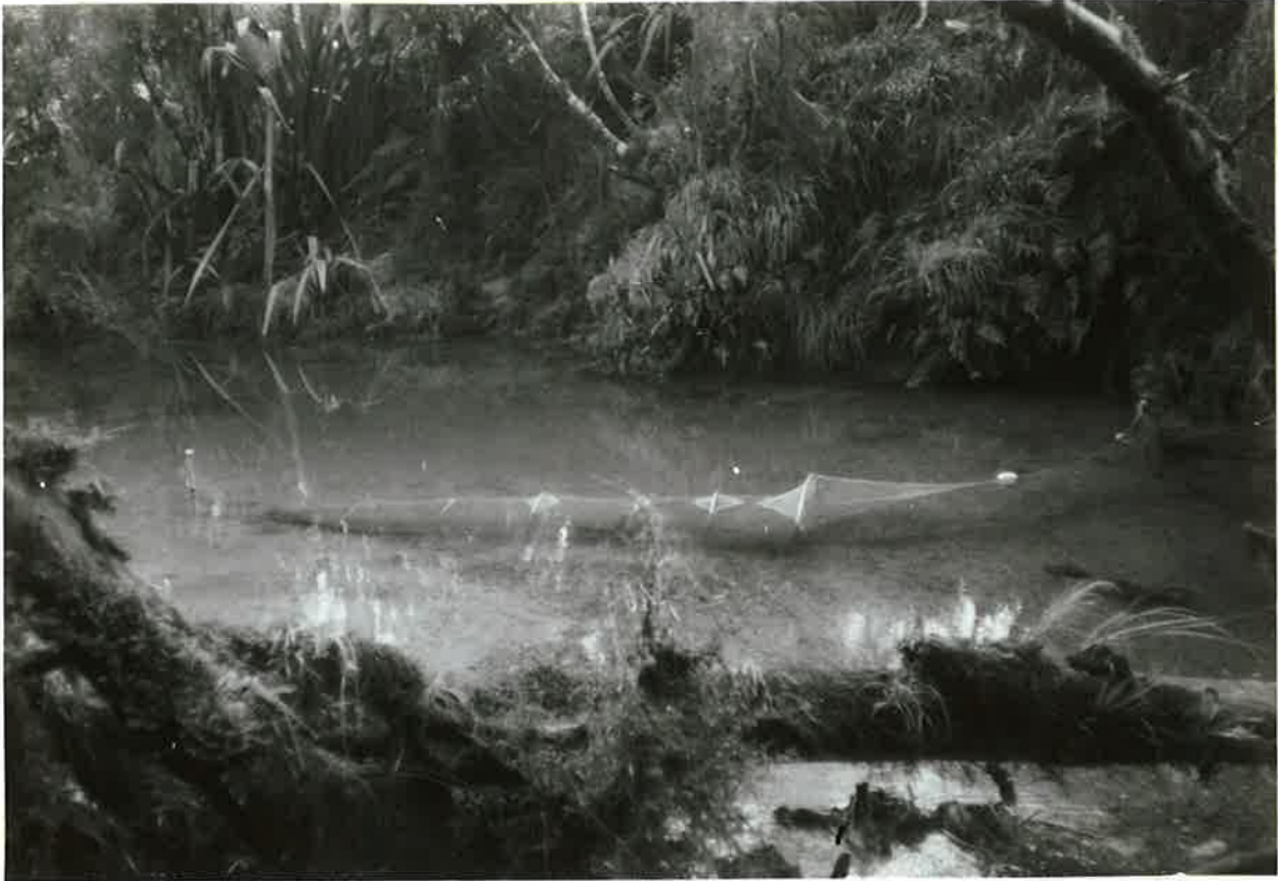
FIGURE 4. A single-wing fyke net set in a tributary of Power Creek (Ohinemaka catchment).
