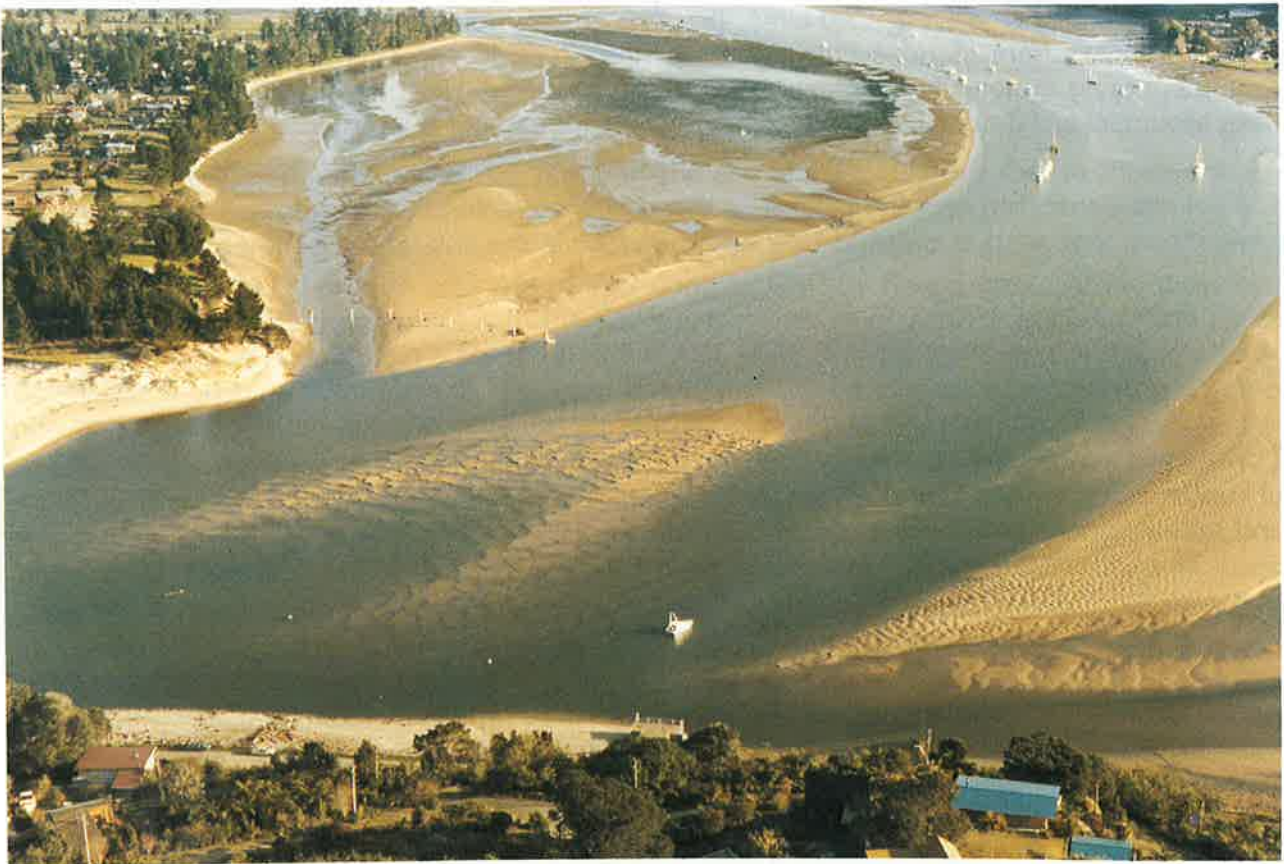
Figure 8: Photograph taken 14 June 1983 at low tide looking southwest from Paku Mountain showing the flood-tide delta partially blocking the main navigation channel into Tairua Harbour.
