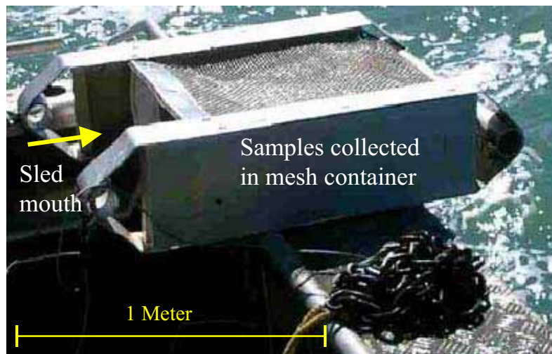
Figure 4 Benthic Ocklemann sled.
