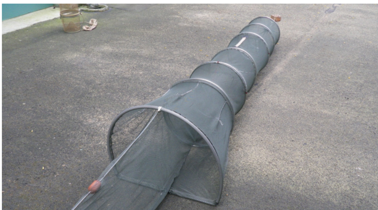
FIGURE 17. Recommended standard fyke net for use in fish sampling of New Zealand wadeable streams.
