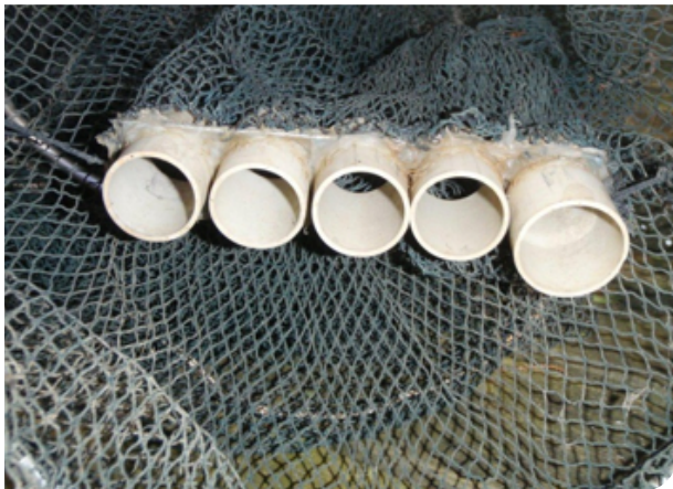
FIGURE 13. PVC separation tubes used in fyke nets during the field trials.
